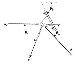
The component of force **F** acting along line *aa* is required to be 30 N. Determine the magnitude of **F** and its component along line *bb*. Given:
